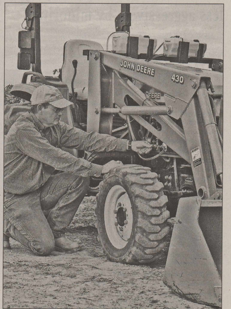
STEVE OSWALT, DOCTORAL student and research farm manager, explains the biodiesel-run tractor, fueled by cottonseed oil, during a national conference concerning alternative fuels at the Crop Research Lab.
