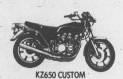
The KZ650 engine is built to deliver the performance of a 750, in a bike with the size and handling of a 550. It has 652cc, 4 stroke with double overhead cams, mag wheels dual front disc and rear disc brake
