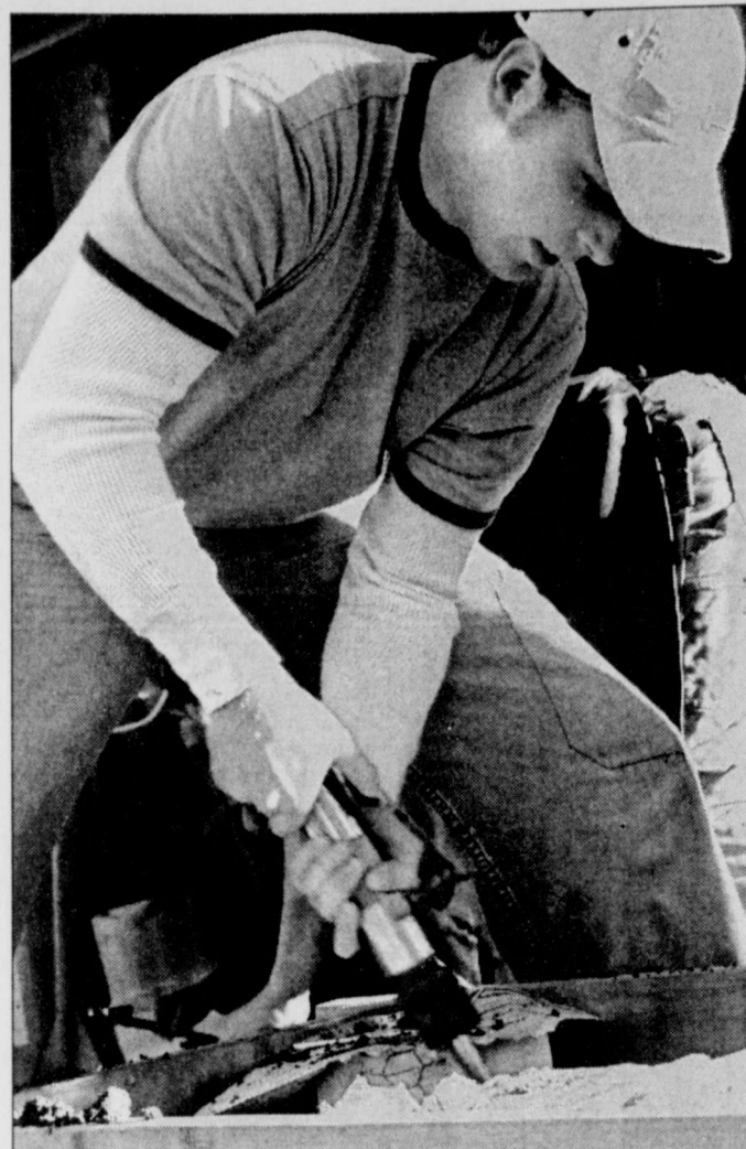
JENNA HANSEN/Staff Photographer BRITT TROLINDER, A graduate student studying mixed media from Quanah, uses a pounder to pack sand against his mold in the Foundry on Wednesday afternoon.
