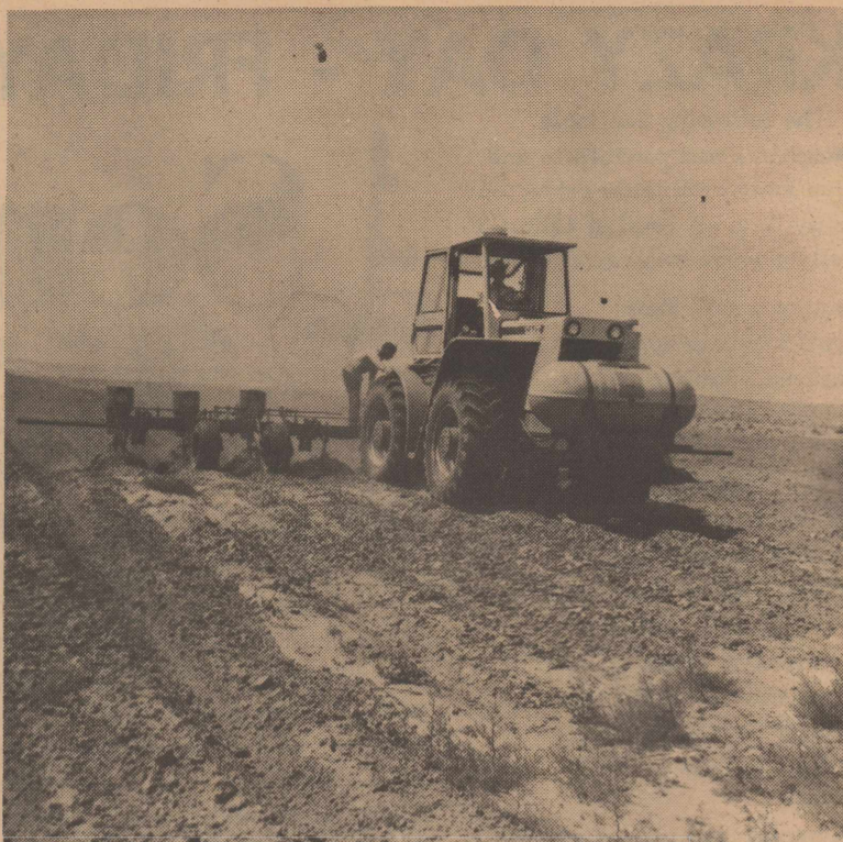
THIS BIG CASE TRACTOR IS PULLING 10 BUSTERS. IT PLANTS 3 ROWS, SKIPS 1 ROW, PLANTS 2 ROWS, SKIPS 1 ROW AND PLANTS 3 MORE ROWS OF MILO. THE OPERATOR, KELLY CORTEZ, SAID HE COULD PLANT 175-180 ACRES A DAY WITH A RIG. HIS EMPLOYER, NELSON CAYTON, ROUTE 3, SEMINOLE, WORKS ABOUT 1800 ACRES.
