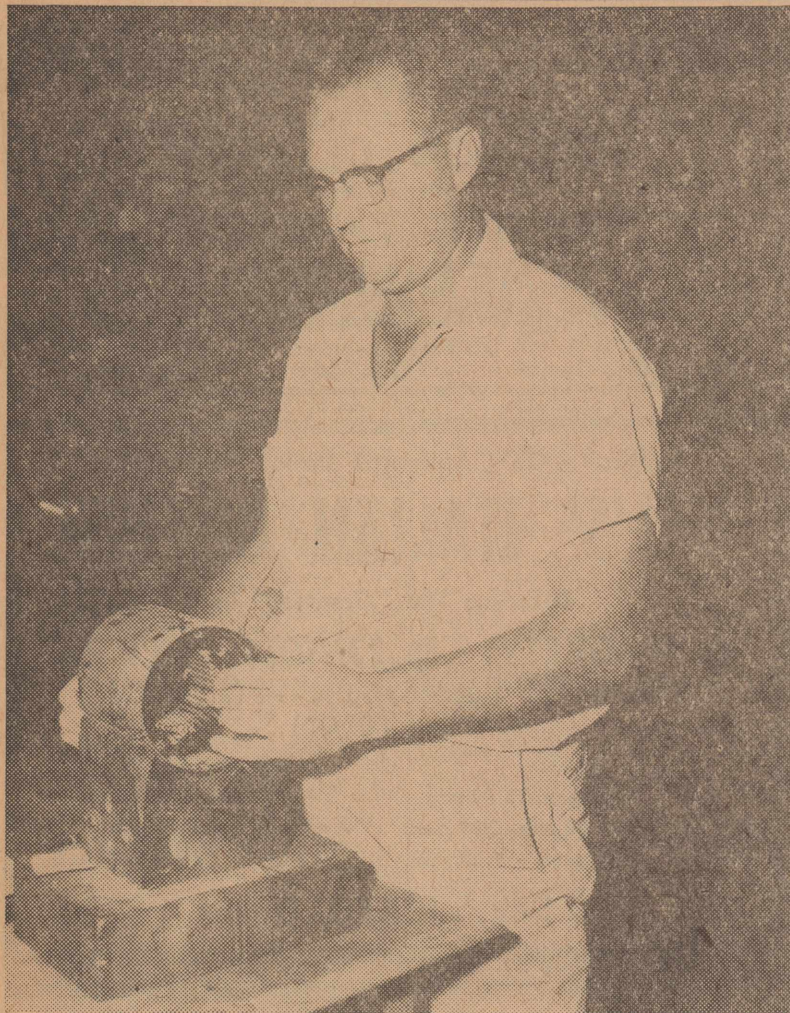
VALUABLE EMPLOYEE — Ward Abbott, one of the base's 108 physically handicapped personnel, rewinds a generator coil in the electric shop in his daily duties. Emphasis is on his work and that of other handicapped employees during observance of "National Employ the Physically Handicapped Week," October 7-14. (Photo by Roca.)
