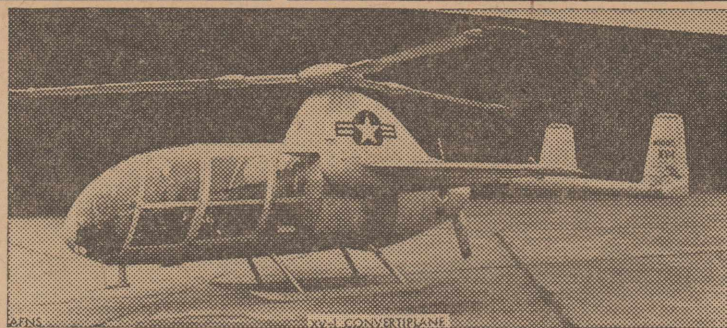
THE XV-1 —The world's first successful convertiplane—recently unofficially exceeded the speed record for helicopters when it reached 200 miles an hour. In tests, the aircraft has made conversions from helicopter rotor take-off to airplane forward flight and back to rotor for landing, the only such plane that has made conversions in flight.
