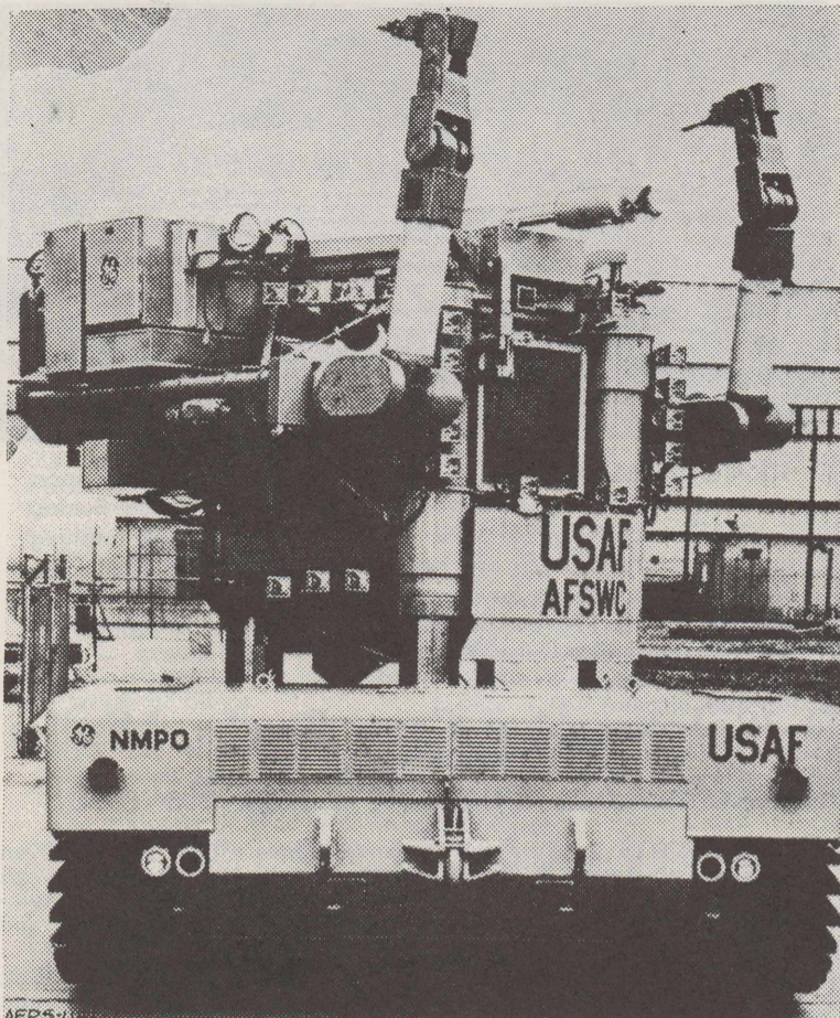
'BEETLE' ROBOT—Built for the Air Force to work in "hot" nuclear environments, this 85-ton robot can rise to 25 feet above ground level and rotate in a circle. Equipped with 16-foot arms and mechanical hands, it is designed to perform assembly or disassembly operations, make adjustments or do emergency duty. Following a six-month testing and checkout program in Nevada in cooperation with the AEC, the Beetle will be used in direct support of the Rover nuclear rocket program.
