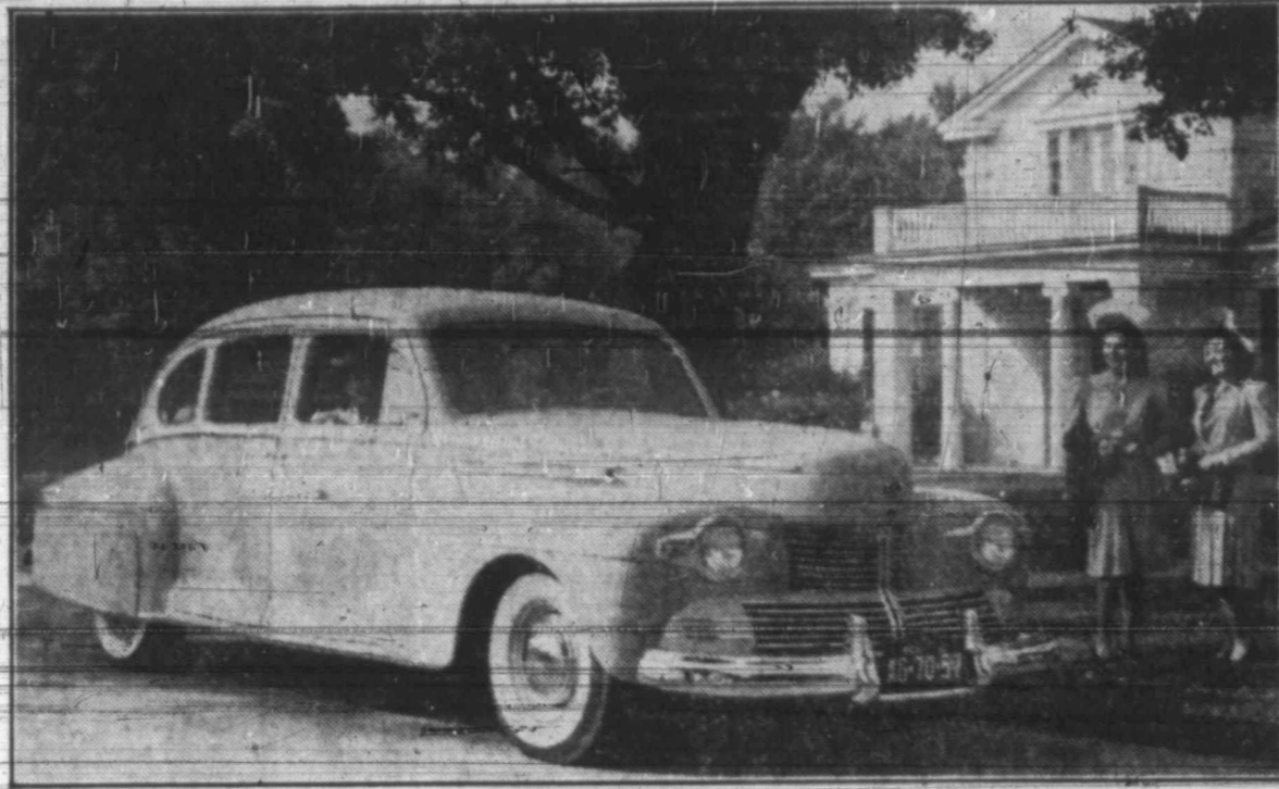
THE LINCOLN LINE for 1942 presents entirely new styling as shown in the Four-Door Lincoln-Zephyr above. Similar style treatment distinguishes the Lincoln-Continental and Lincoln-Custom series. Broad grilles of rustless steel emphasize the reduced overall height of the bodies as do the long, widely flared fenders. Door handles are replaced inside and out by flush-type push-button latch controls which are employed also on the locks of the luggage compartment. The new cars are on display at Bennett Motor Co., 1008 Avenue J.
