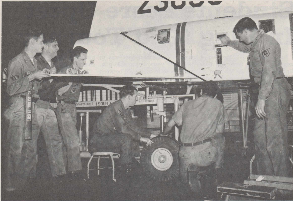
DOCK CREW —Members of Dock Three, the Dock Crew of the Month from the T-38 maintenance section, install the tail section on a Northrop T-38 Talon aircraft. The crew was selected for having the least amount of discrepancies during September in processing seven aircraft. Members of the crew are, left to right: Sgt. James Baer, A1C Michael Blair, Sgt. Richard Woods, Sgt. Paul LeBlanc, A1C Timothy Duncan, Sgt. Larry Wright (hidden) and TSgt. Dale Burton, dock chief. (U.S. Air Force Photo)
