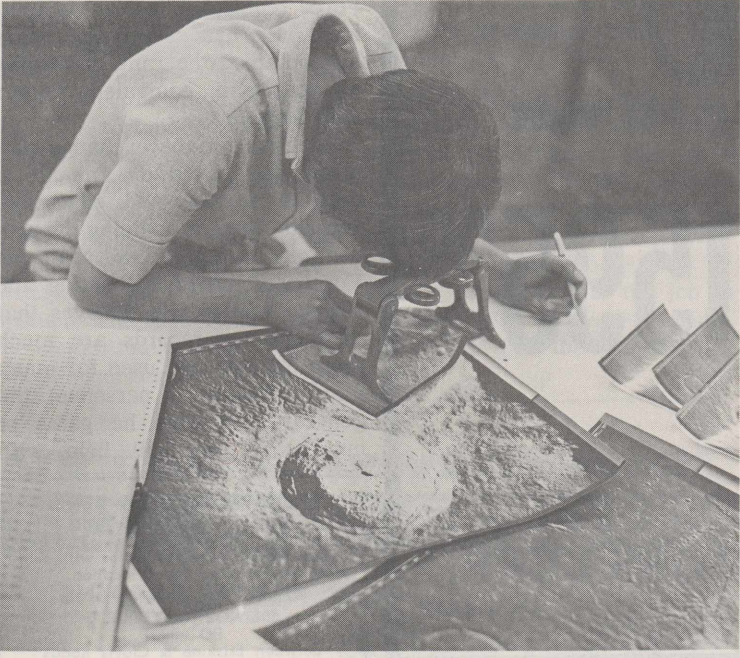
SEEING MOON—Looking through a stereo viewer, Miss Sue Doi of the U. S. Air Force Aeronautical Chart and Information Center Astro Charting Branch views the moon in 3-D. The stereo viewer permits the operator to view the lunar photographs in simulated three-dimensional format thus allowing for better photo interpretation. (U.S. Air Force Photo)
