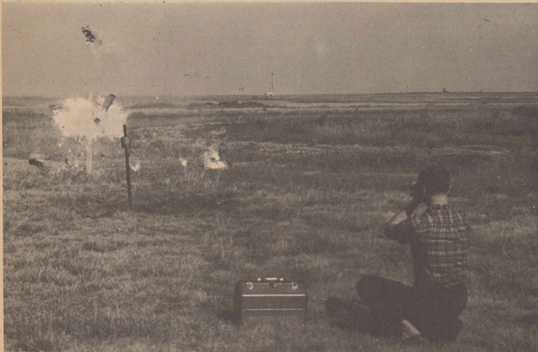
LIQUID OXYGEN — A cameraman from KCBD-TV, Ralph Shelton, was on hand Tuesday morning to film the liquid oxygen demonstration given by a ground safety team from Sheppard AFB. The team detonated a liquid oxygen and hydrocarbon 'gel' inside a flight suit to demonstrate the dangerous nature of the compound.
