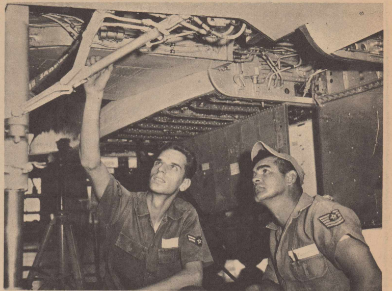
INSPECTION — TSgt. James H. Montgomery, a dock chief with the 3500th Organizational Maintenance Squadron checks the hydraulic landing gear system of a T-38 after A2C Wallace E. Parry Jr., a member of the sergeant's crew, called his attention to a possible leak.
