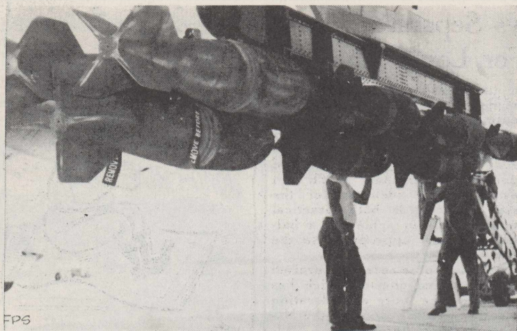
LOADING UP —Ground crewmen load 750-pound conventional bombs under the wings of an Air Force B-52. The operation was part of recent tests of SAC's capability to deliver conventional weapons at the Air Proving Ground Center, Eglin AFB, Fla.
