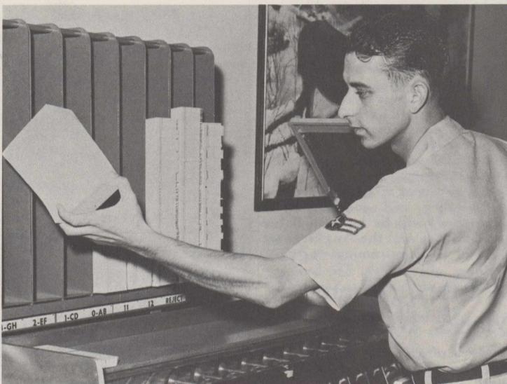
CARD SORTER — A2C Gary Richardson stacks data cards in an 84 type sorter as an early step in preparing more than 500 reports a month for Reese.
