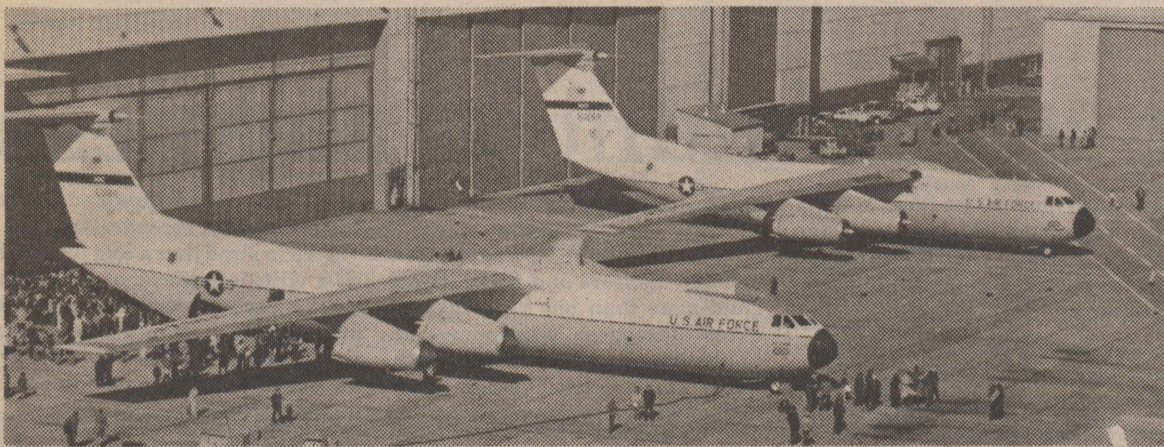
EXTENDED STARLIFTER - Dubbed the YC-141B, this "stretched" C-141 is 23 1/3 feet longer than the standard C-141 in the background and can carry some 13,000 pounds more cargo. The experimental aircraft was rolled out recently at the Lockheed-Georgia plant near Dobbins AFB, Ga. (U.S. Air Force Photo).
