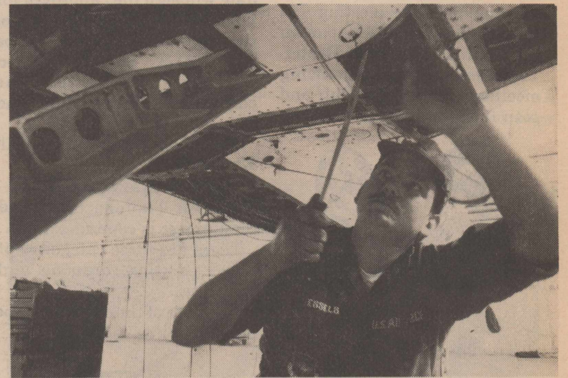
A1C Rick Wessels works to disengage a wing from a T-38 Talon trainer. The base will replace a wing on another T-38, one of the aircraft whose wings the Air Force has found to fall below accepted standards for fracture toughness. (Photo by Ted Houghton)
