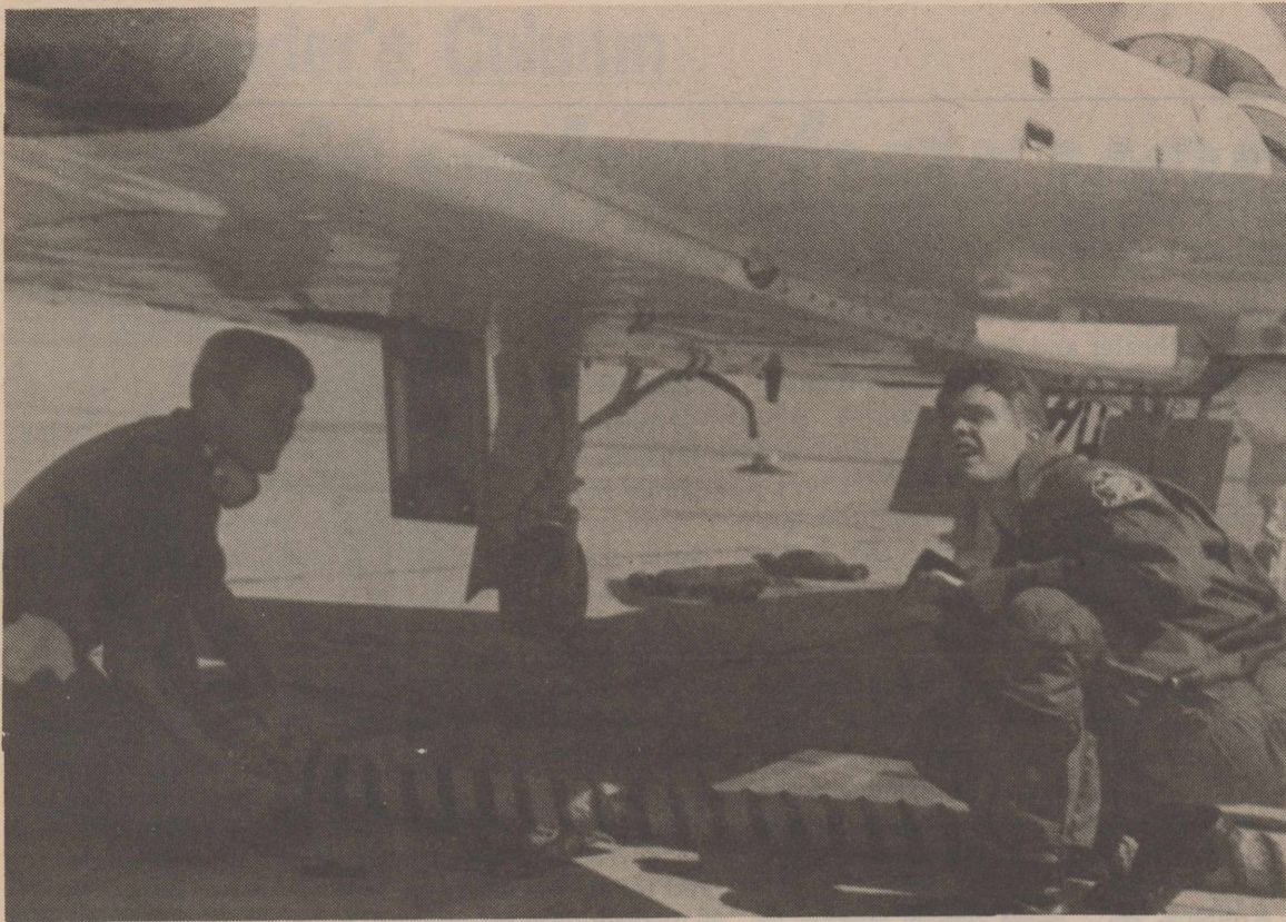
Staff Sergeant Larry Close (left) hooks up an air starter hose while he prepares a T-38 for launch as 1st Lt. Mark Butorak does a pre-flight check prior to his flight. Sergeant Close is assigned to 64th OMS Fox Flight, and Lieutenant Butorak is assigned to 54th FTS P-QUAL.
