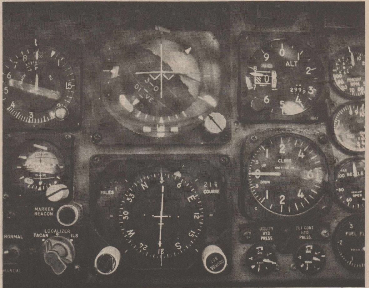
Air Force pilots are trained in the T-crosscheck for instrument flight. The change to multi-function and head-up displays in newer cockpits means the pilot takes longer to read specific numbers than with the analog (round dial) instruments. (U.S. Air Force photo by SMSgt. Ron Scharven)
