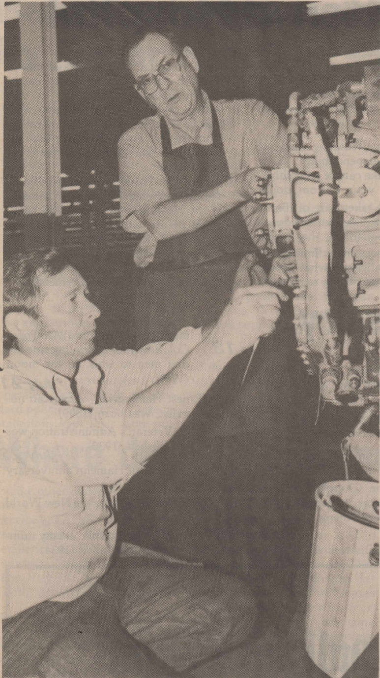
Charles Nance (top) and Virgil Holt take off an accessory case of a J-69 engine in the 64th Field Maintenance Squadron engine shop. During the last few weeks, the J-69 Engine Shop reported that all 156 T-37 engines were serviceable, which included all 11 spares. No one recalls having a 100 percent spare line here at Reese before.
