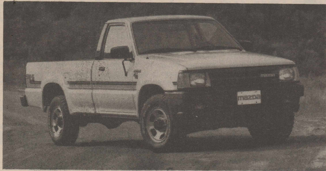
HIGH RIDING STYLE —All Mazda B2600 4 x 4 models, including the SE-5 (above) and Standard (below), have 8.2 inches of ground clearance, which comes in handy when the off-roading gets rough. Standard skid plates on the oil pan and transfer case help protect the undercarriage from rock damage.
