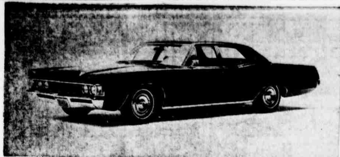
ROOMIER, LONGER and completely new, the Mercury Monterey for 1969 offers a full range of nine models in the Monterey and Monterey Custom series. They are 221.8 inches long, an increase of almost two inches. Roadability is improved, with wheelbase increased to 124 inches and tread wider in front by one inch and in the rear by two inches. Interiors reach a new level of luxury, convenience and comfort. The new body features cleaner lines, smoother contours and the long-hood short-deck design characteristic of the Continental. Pictured above is the Mercury Monterey Custom four-door sedan.
