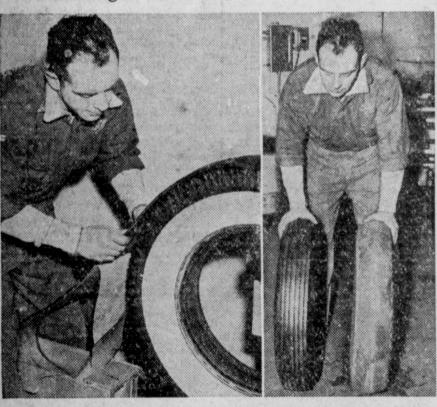
We will all have to do without new automobile tires for the present. Next best thing is a retreading job on your old ones, if they are too smooth for safety. At left you see a re-treading operation in progress. A "camel back," or new rubber top, is vulcanized to the old casing to give a new gripping tread. At the right is shown how a worn-out tire compares with one that has just been given a face lift, or a new tread. The recapped tire is at left; the old "smoothy" beside it.
