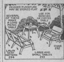
The construction is so simple that all you need is stock widths of lumber, a hand saw, a screw driver and a brace and bit to bore the holes for the pegs.
