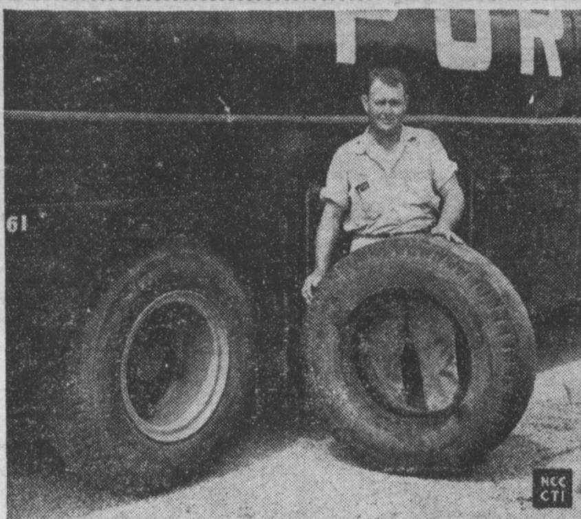
This sturdy veteran from a group of tires tested for performance with a fleet of heavy gasoline trucks has given 100,000 miles of service its cotton cord carcass outlasting three recappings. Made under identical conditions with the same amounts and types of rubber, but using different fibers in the cords, the tires showed different degrees of stamina. Rayon cord tires lasted for an average of 25,985 miles, cotton cord tires for averages of 46,399, 50,673 and 50,975 miles. Admiring the tire in the picture is Sam Lazenby of Hughes, Ark., himself an oil company distributor.
