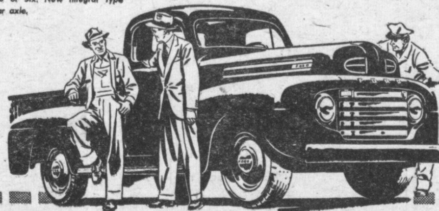
Ford 6 1/2 ft. half-ton Pickup, G.V.W. 4,700 lbs. Choice of two engines, V-8 or Six. New integral type rear axle.
