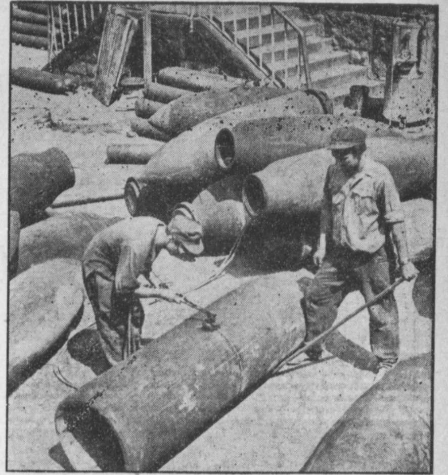
LEFT OVER FROM THE BLITZ —Workmen in Berlin use an acetylene torch to carve up a two-and-a-half-ton blockbuster for scrap. Originally destined for England via the Luftwaffe, the bombs are among hundreds of tons of scrap iron and steel being shipped daily to England by a more peaceful water route.
