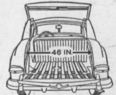
Only Kaiser Traveler has a cargo hatch that swings open clear to the roof, with 46 in. minimum width, and 38.6 square ft. of steel-shod deck space in the cargo hold.
