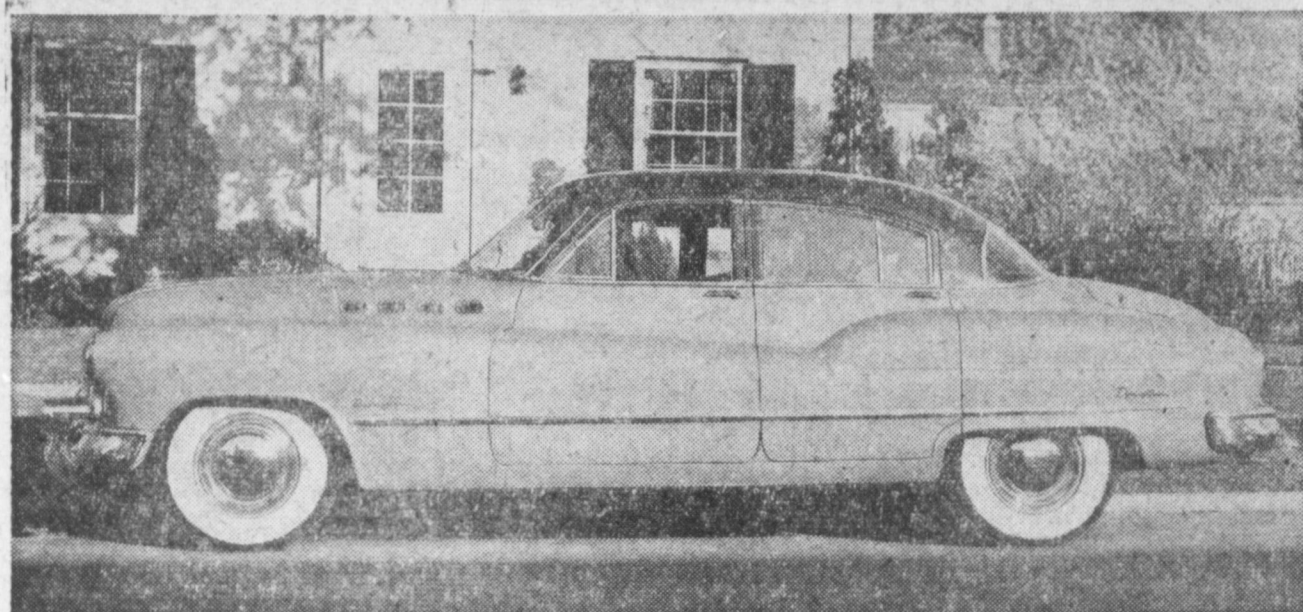
Tops in the Buick line for 1950 is the stately Roadmaster six passenger sedan. Inches shorter than its predecessor the car has a more powerful engine, a completely new body and features a one-piece curved windshield. Note the full taper-through of the front fenders, the wrap-around bumpers, spacious trunk and the narrow rear quarter panel permitting the rear window to come well around to the side providing better rear vision for the driver.
