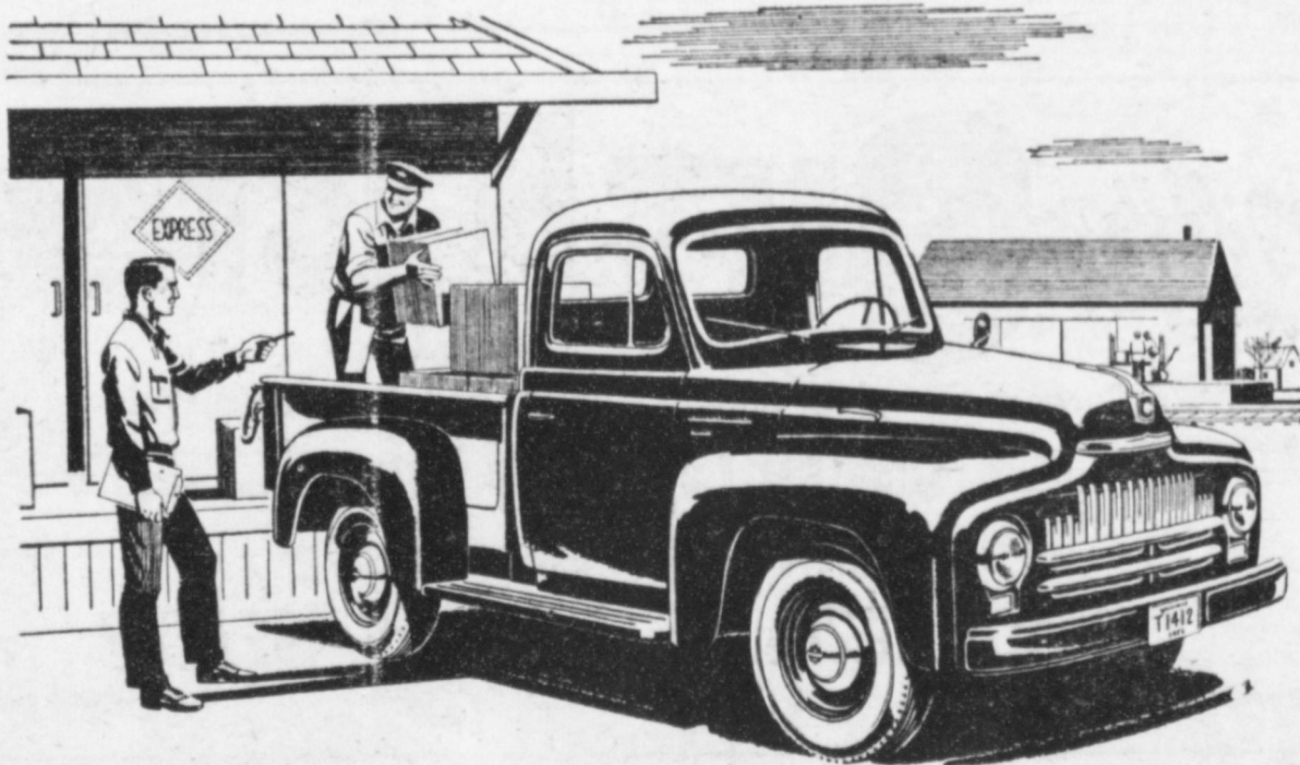
Model L-110, 115-inch wheelbase, 6 1/2-foot pickup body, 4,200 lbs. GVW. Pickups in the L-110, L-120 and L-130 Series include 115, 127 and 134-inch wheelbases, 6 1/2, 8 and 9-ft. bodies, GVW's to 8,600 lbs.
