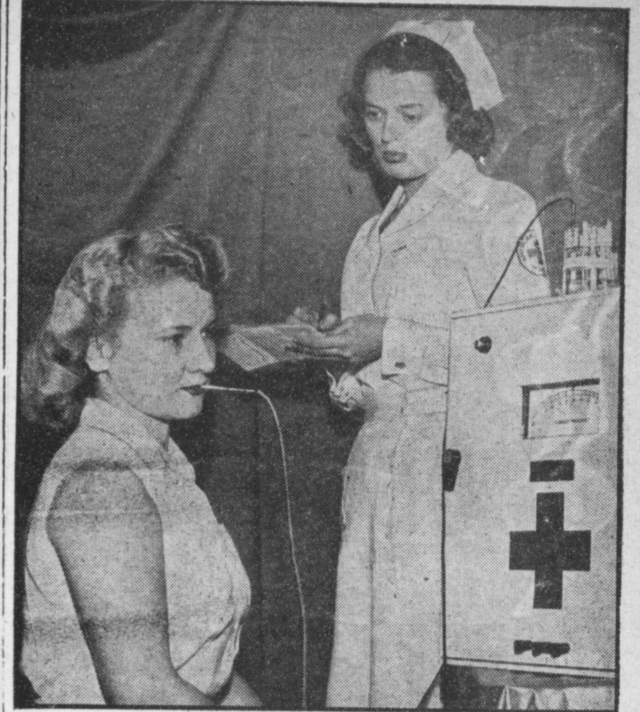
ELECTRONIC TEMPERATURE TAKER —A newly developed electronic thermometer takes temperatures twice as accurately as the old fashioned thermometer and 60 times as fast. Waiting the few seconds necessary to take a reading is pretty blond Philadelphia blood donor, Arlene Delaney. Ready to write the figure down is Red Cross Nurse Mary Douglas. Developed by Minneapolis-Honeywell engineers, the device will speed up blood donation time in case of disaster when many donations must be taken quickly.
