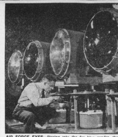
AIR FORCE EYES-Staring into the far blue yonder, these four unblinking airport beacons are getting final adjustments before being sent to Air Force bases. Manufactured by Westinghouse Lighting Division in Cleveland, Ohio, the 3,000,000 candlepower beacons are 24 inches in diameter and can be seen at a distance of 50 miles.
