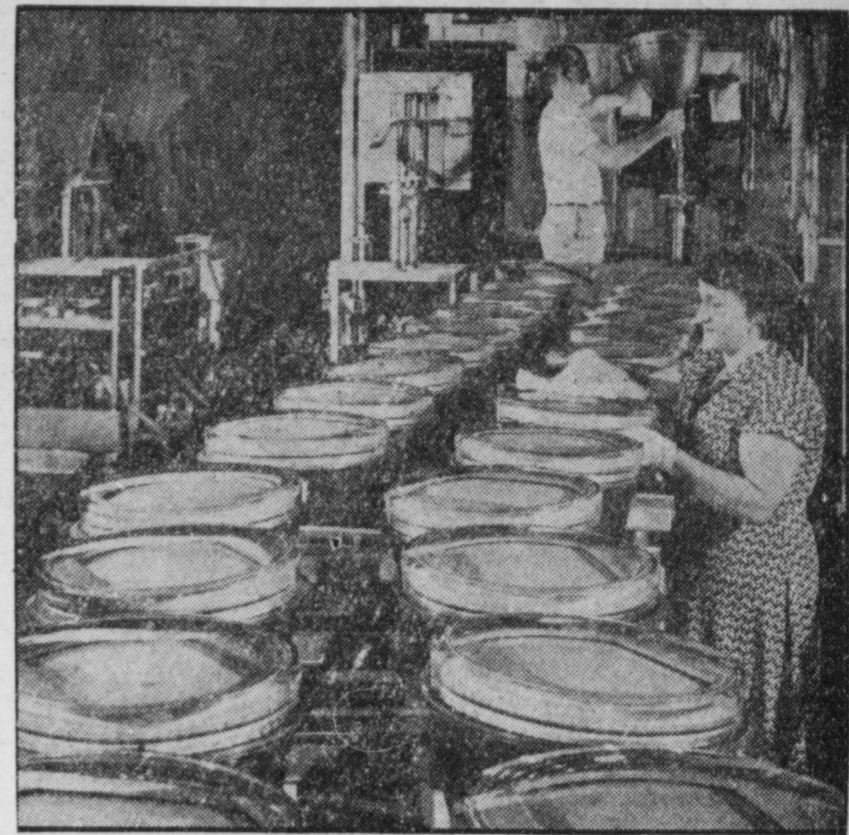
COLOR COMING —Only the go-ahead signal from Washington is needed to add color to television. Proof that color TV is just around the corner is this assembly line of color tubes at the Lancaster, Pa., RCA plant. These tubes are about to undergo an "exhausting" experience as they move toward the air-exhausting machine which creates a near-vacuum within the tubes to assure successful electronic operation.
