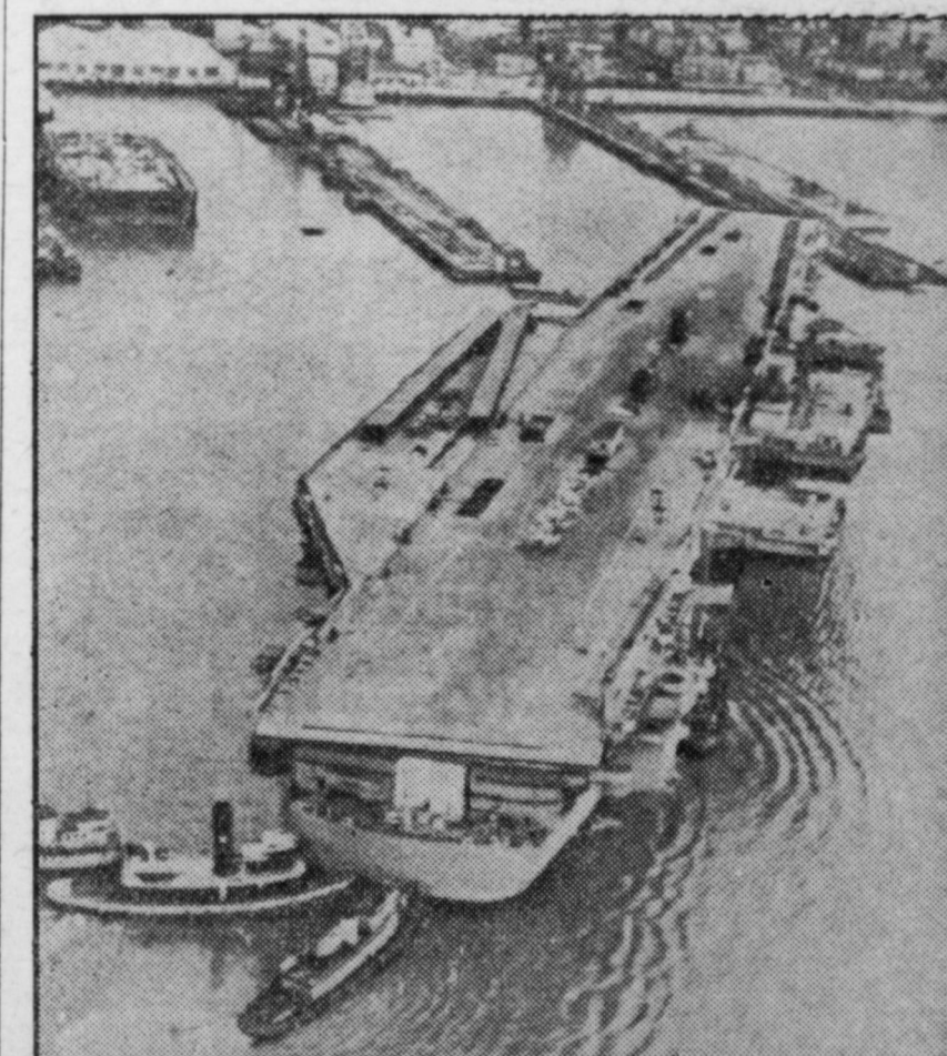
OPERATION NUDGE —The USS Forrestal, world's mightiest warship and largest ship ever constructed in the United States, is nudged by tugs into an outfitting dock at Newport News, Va., following her christening. Vital statistics: Overall length, 1036 feet; extreme breadth at flight deck, 252 feet; over 200,000 horsepower; a rated speed which tops 30 knots; nearly four acres of flight deck; height from keel to top of mast equals height of a 25-story building; crew of 3500 needed to man her.
