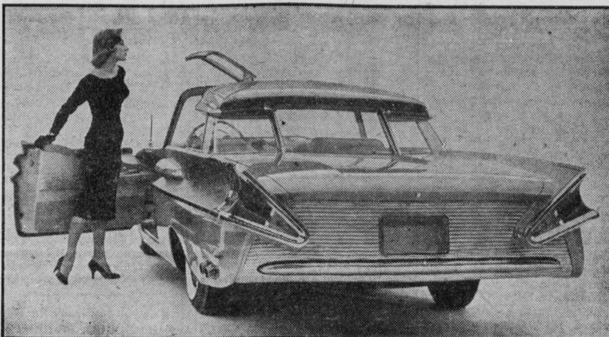
GEARED TO TOMORROW —Scoop-channel sidewalls and fenders, "butterfly" roof inserts which raise as doors are opened and turn-and-stop lights at left and right-hand corners of roof mark the striking design of Mercury's experimental XM-Turnpike Cruiser. Only 4.4 feet high, the car is styled to meet roll across the nation's ever-expanding highway system. Other features: Side-vent exhausts beside left-rear wheel and windows which wrap around corners usually occupied by frame posts. First shown in Chicago, the machine will be put on a nationwide display tour.
