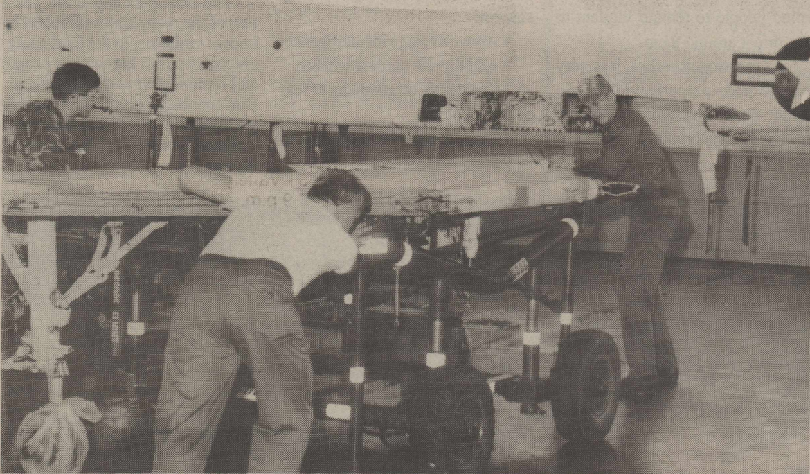
(L-R) SSgt. Stephen Ulrich, Sgt. Eugene Adkins, and Sgt. George Kostelnik, all assigned to the Aero Repair Branch of the 64th Organizational Maintenance Squadron, are shown removing a T-38 wing as part of the wing radius bushing inspection. The inspection procedure is exacting, tedious and time-consuming, but it is another example of the professional maintenance performed to the highest standard by the Aero Repair Branch. Wing radius bushings must be inspected after every 2700 hours of flying time. (USAF photo)
