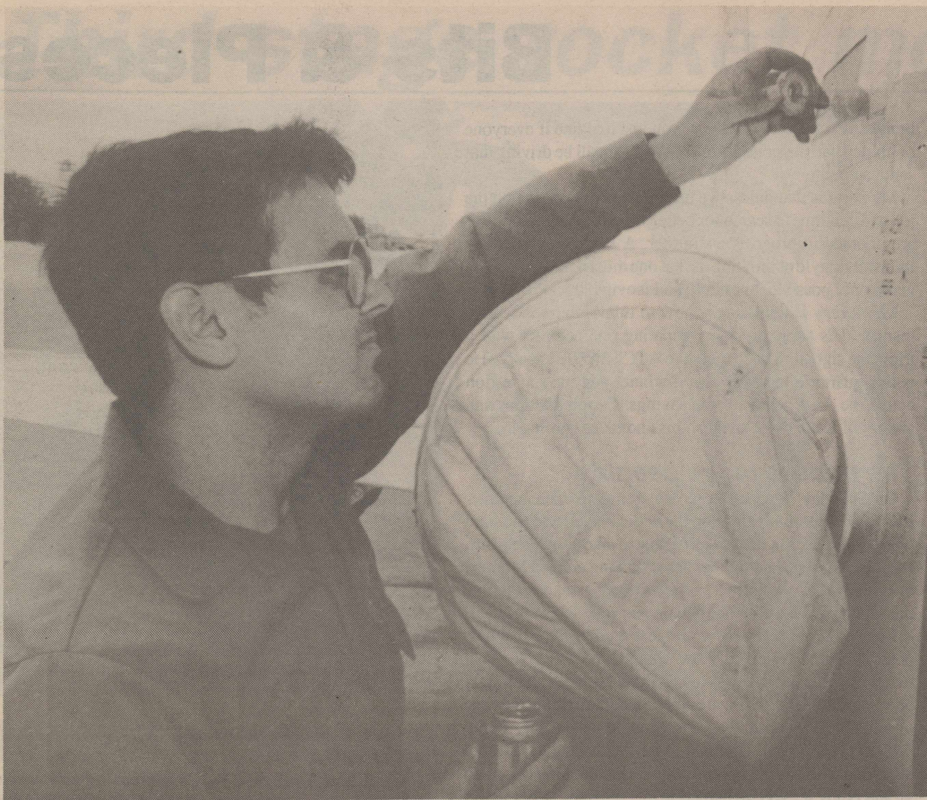
TSgt. Kenneth Brown, Assistant Flight Chief, 64th OMS Eagle Flight, glues stickers on a recently painted panel. The panel, a composite material being tested by Northrop Air Division, will be used on 18 of Reese's T-38 for the next two and one-half years. (USAF photo)
