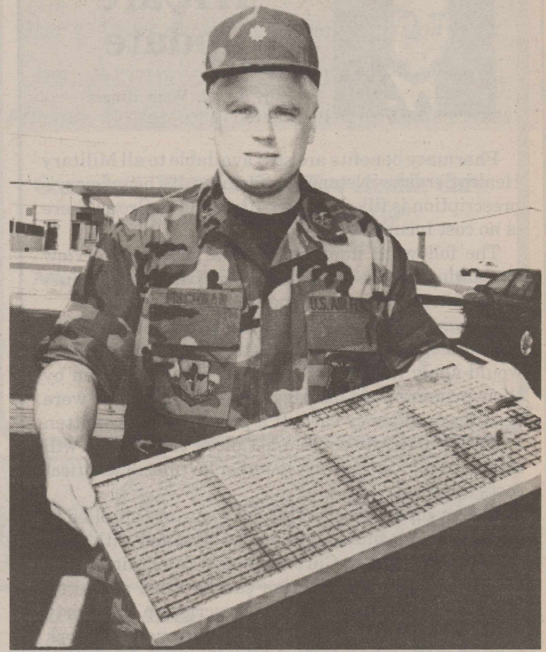
Maj. Len Fischman holds a dirty air filter responsible for causing carbon monoxide poisoning.
