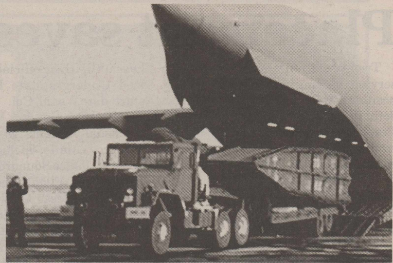
A M172A1 mobile bridge, used by armored vehicles to cross bodies of water, is pulled off a C-17 Globemaster III during an engine-running offload at Tazsar airfield in Kaposvar, Hungary. Secretary Perry says the C-17 is proving its worth daily.
