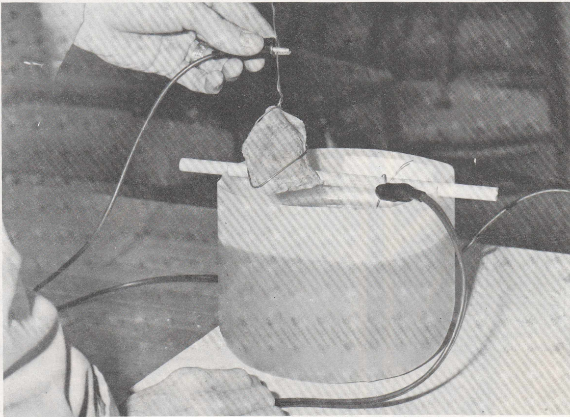
Mike Thornton prepares to dip a metal matrix into an electroforming bath.
