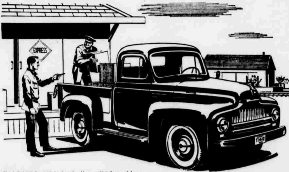
Model L-110, 115-inch wheelbase, 6 1/4-foot pickup body, 4,200 lbs. GVW. Pickups in the L-110, L-120 and L-130 Series include 115, 127 and 134-inch wheelbases, 6 1/4, 8 and 9-ft. bodies, GVW's to 8,600 lbs.
