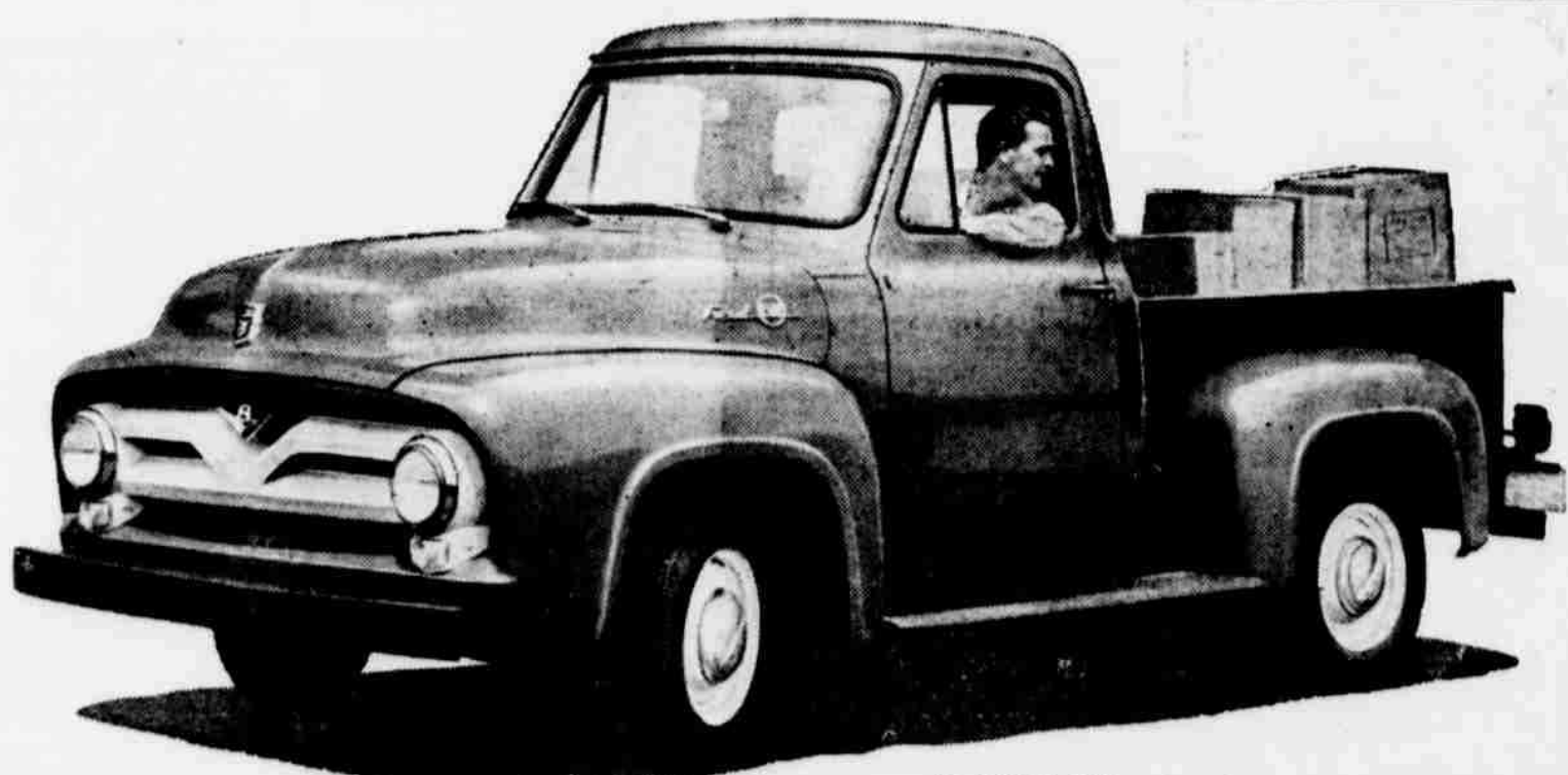
Ford 6 1/2-ft. Pickup gives choice of Short Stroke 132-h.p. V-8 or Short Stroke 118-h.p. Six. Tubeless tires standard. Fordomatic Drive and Power Brakes available at low extra cost. GVW 5,000 lbs.
