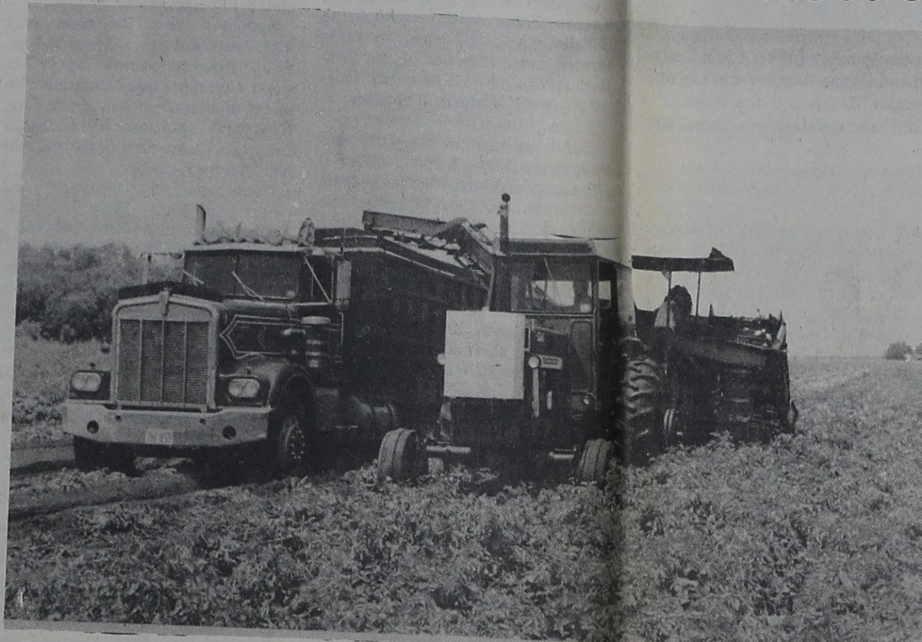
POTATO HARVEST in action is shown here as the field of Tacho Ramirez west of town is emptied of its crop. A conveyor belt carries the potatoes from the mechanical picker to the truck. Digging operations are in full swing this week as skies cleared up and the ground is dry enough to make the job a little easier. It is hoped that plenty of potatoes will be ready for sale at the Knox County Vegetable Festival June 18.
