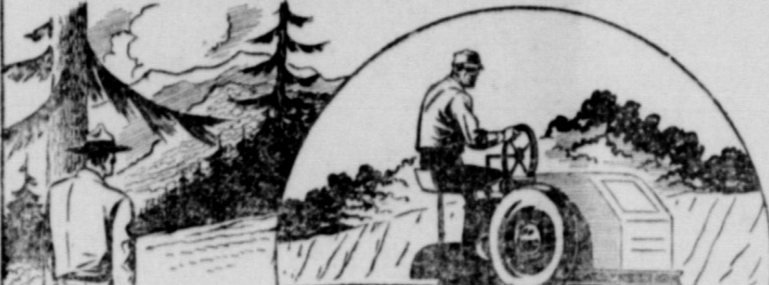
AIRPORT REPAIRS AND ROAD PATCHES CAN BE COMPLETED QUICKLY WITH THIS NEW HIGHWAY ROLLER WHICH IS EQUIPPED WITH RETRACTABLE PNEUMATIC TIRED WHEELS FOR QUICK MOVEMENT FROM ONE PLACE TO ANOTHER
