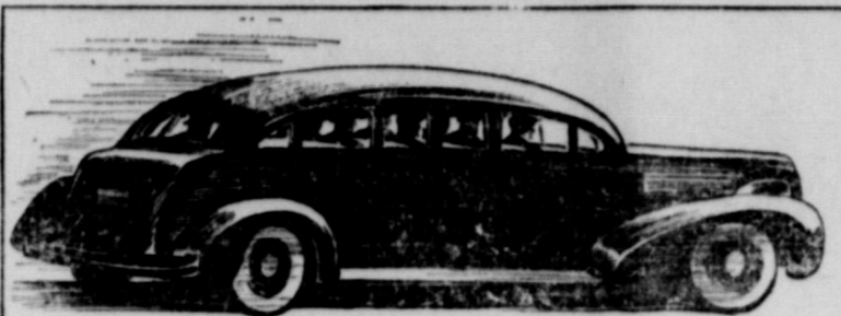
A 15-PASSENGER GAS-AND-RUBBER-SAVING CAR IS BEING MADE FOR WAR WORKERS. A FOUR DOOR SEDAN IS CUT IN HALF, AND A SIX-FOOT EXTENSION INSERTED IN THE MIDDLE
