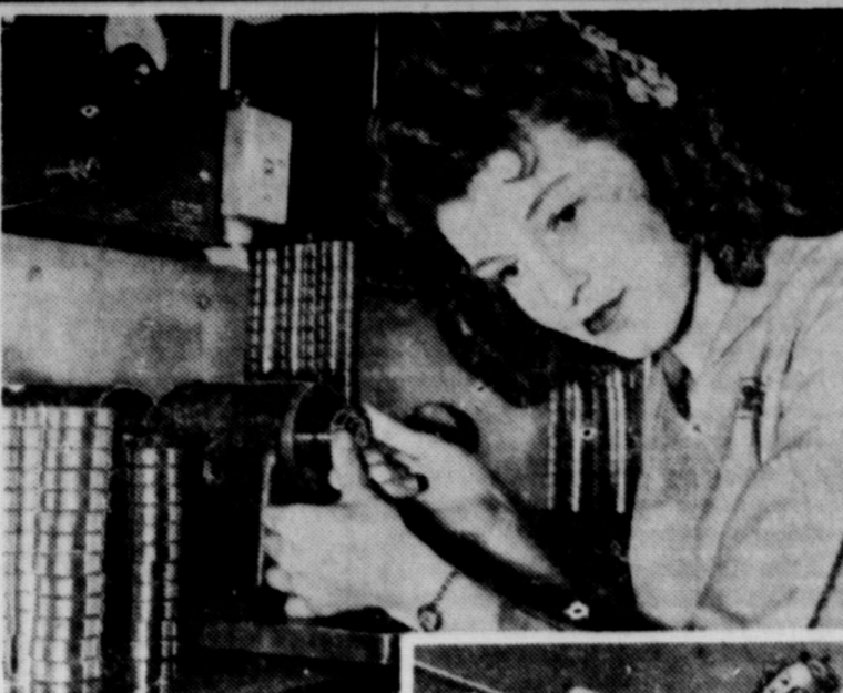
A-CUTE EAR —Specks of dust or invisible scratches can cause noise in precision-made ball and roller bearings rotating at high speed. Here Colleen Nevrousky, testing expert at SKF Industries, Inc., Philadelphia, listens through magnifying apparatus to decide whether bearing will pass or be rejected.
