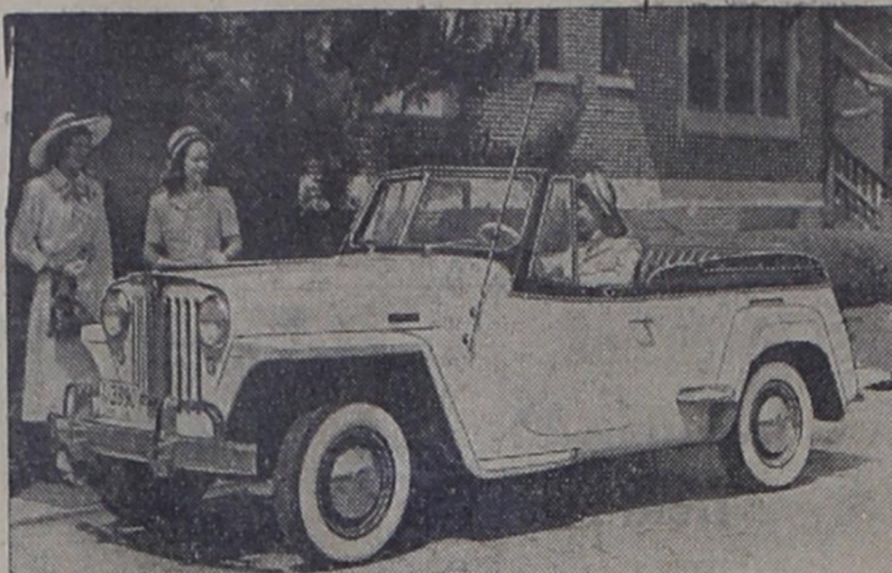
The latest member of the Jeep family is Willys-Overland's newly unveiled sports phaeton, the Jeepster. Styled in the continental fashion, the car is a glamorous, smooth-riding descendant of its rugged forbear and is one of the first full-sized light cars to appear on the market. It is powered by the Jeep engine, and has independent front wheel suspension. The Jeepster weighs only 2500 pounds, gives as much as 29 miles to a gallon and has a low center of gravity for roadability. Willys-Overland calls it "a sun car built for fun."
