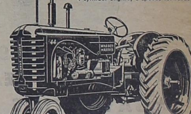
3-4-Plow "44"—260-cubic-inch, 4-cylinder engine, 5 speeds forward.
