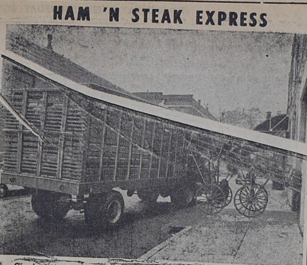
Cincinnati, Ohio . . . Cattle and hogs get a one-way ride from Cincinnati's Central Market to the plant of J. & F. Schroth Packing Company in a Fruehauf livestock trailer. The vehicle is easily maneuvered through narrow city streets because the trailer turns in the same radius as the small truck which pulls it.
