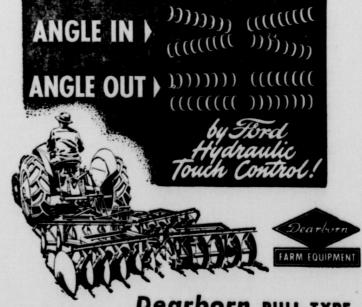
Control lever on the Ford Tractor. Then when you push the lever down the gangs take this angle. When you move the Touch Control lever up, gangs become straight . . . for easy fuel-saving turns, protecting grassed waterways or pulling through wet spots.
