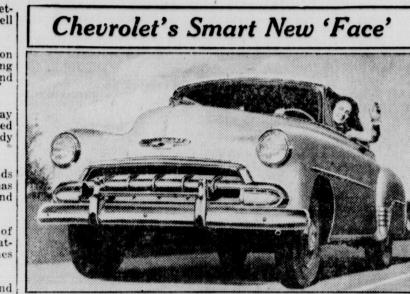
Marked changes from previous years give the 1952 Chevrolets a freshness that assures their continued popularity in the low-price auto-motive field. Apparent in this front-end view is the redesigned grille which features five distinctive "air foil" fins mounted on the center bar. Parking lamps have been broadened to eliminate the former slotted grillework and the hood emblem carries the name, Chevrolet.
