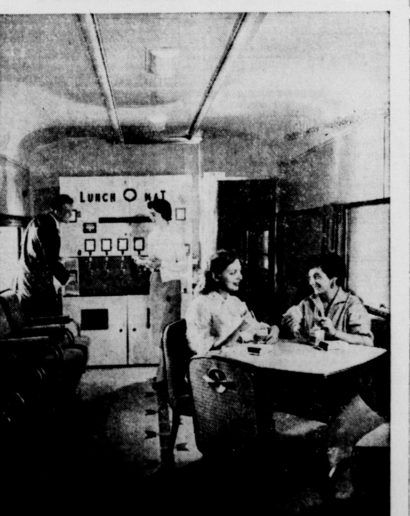
A coin-in-slot device offering hot or cold sandwiches, assorted pastries, fruit juice, milk and coffee, is a new service for Santa Fe Railway passengers. The only one of its kind installed on any railroad, the Lunch-O-Mat uses radar to heat sandwiches in 10 to 14 seconds. This service is initially being inaugurated on a new Albuquerque to El Paso train.
