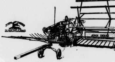
Deere Binder we use an adjustable boxing, with ground bearings. The advantage in this is that you can take up the wear, which is bound to come sooner or later, and in addition the grinding of the bearings makes a much more perfect fit.
